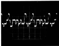
Fig. 6 MIXTURE OF 3 FREQUENCIES WITH PRESET AMPLITUDES.
